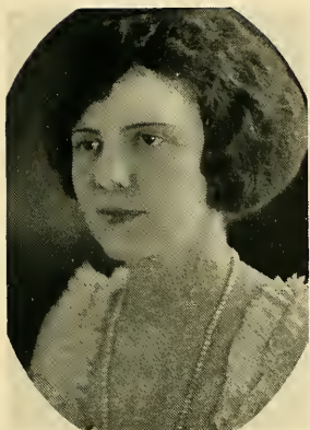
Square finish halftone made from an oval photograph. Note the bad effect at corners where parts of the cardboard had to be left in the engraving.
